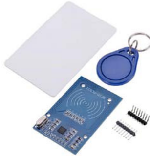
Figure 3.2. RFID module MIFARE RC522 + keychain + keycard (Courtesy of AliExpress)
